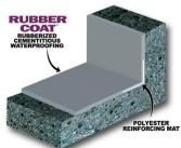
4. Place **Polyester Reinforcing Mat** on concrete corners, 0.3 meter overlapping.
